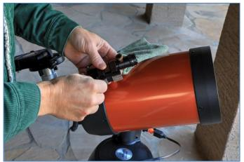
**Remove Tape Film**: Remove the film covering the mounting tape at the front and back bottom of the finder.
