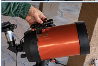
**Fine Tune Alignment**: Ensure the target is still centered in the telescope and make adjustments of the laser using the adjustment nobs to aim the laser at the target.
