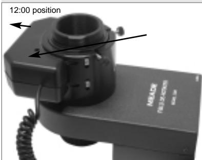
Fig. 59: Place the microfocuser over the adapter ring. Notice the orientation of the microfocuser.
