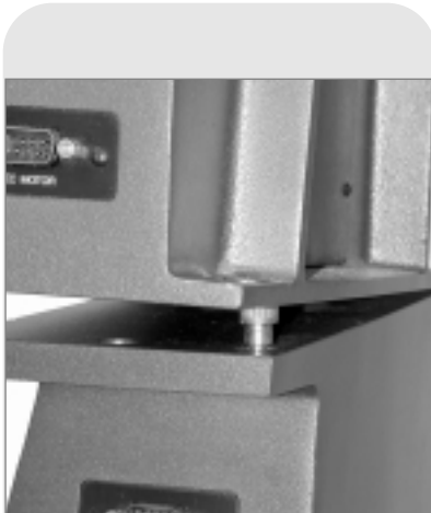
Fig. 52: Position the holes over the shoulder bolts. When they are in place, slide the OTA back so that the shoulder bolts lock into the slots.
