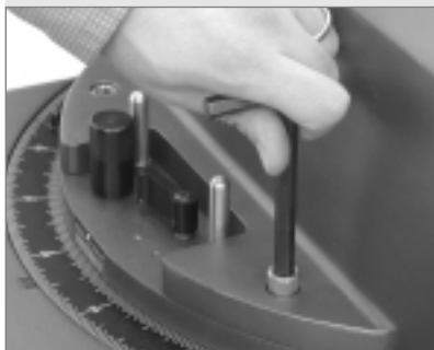
Fig. 49: Bolt the fork to the drive base.
