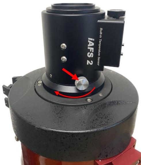
4. Tighten the Locking Screw to lock the focuser. Release the Locking Screw to adjust the focuser angle. Finally tighten three Position Screws after angle adjustment.
