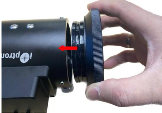
Thirdly, thread 3 Position Screws all the way in, then back out a quarter turn or so. The OTA adapter can be rotated freely but can not be pulled out from the focuser body.
