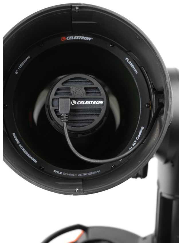
FIG 29: The flat frame taken at the factory and pre-loaded onto Origin was captured with the camera in the orientation shown. If you rotate the camera from this orientation, you'll need to produce a new flat frame.
